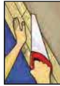
Picture 1: Before installing the first row, the part of the groove profile which sticks out must be cut off.
